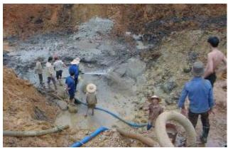
[Tan Huong, Vietnam, ruby and spinel mine. Back hoes remove about six feet of soil then high pressure water is used to loosen the old buried stream bed so the miners can use screens and sluices: Image courtesy of www.gemsfromearth.com]
